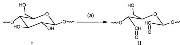
*Fig. 1: Oxidation of cotton (a) [6]*
